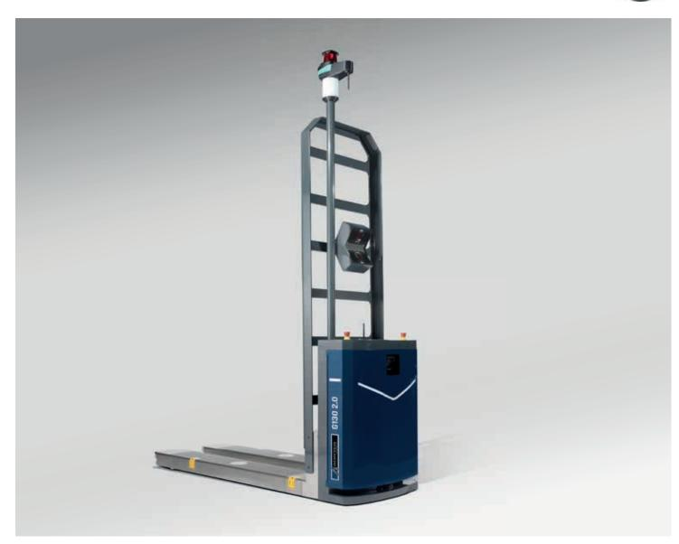
Fully automated loading, unloading and transport of pallets is a task for the smart AGV pallet carrier by A1 Sorter. The G130 Gen 2.0 is a combination of hi-tech with attractive design.
