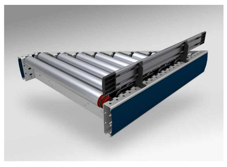
24V conveyors are driven by electric rollers connected by means of multi V-belts with other rollers. The design of this type of equipment allows it to be configured with other systems such as gravity conveyors, belt conveyors, transfers, switches and pop-up modules.
