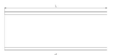
Blend is a cover made of PVC, whose task is to hide and protect the electrical installation located within the devices. In addition, it affects the aesthetic appearance of conveyors. Blends are available in three colors, and their length depends on the order.
