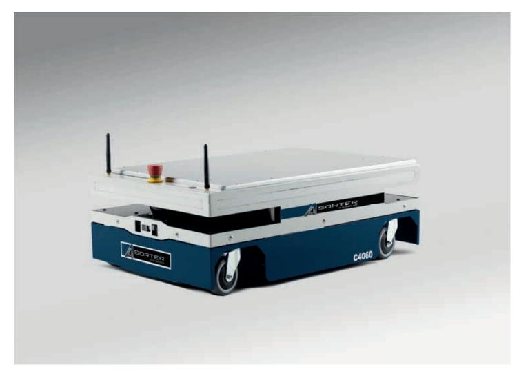
A1 Sorter C4060 is a small-sized (40x60x21cm) smart AGV platform with just 29 kg of weight.
