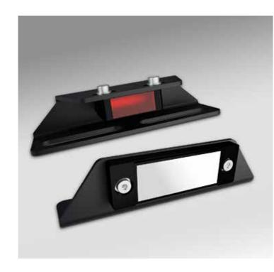
Sensors detect objects on conveyors and determine their location. They are installed on the conveyor frame together with a reflection mirror that reflects the impulse from the sensor. The kit includes a sensor with a cable and a handle.
