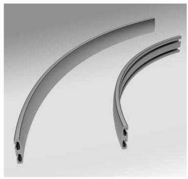
The curved band is used to protect the transported product from slipping off the conveyor line. Profiles are matched by rolling on sections of curves, connecting nodes, and changing direction to ensure the correct flow of cargo. We offer the bands in an aluminum version. The top edge of the band is 90 mm above the conveyor.
