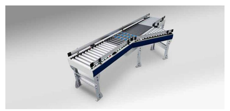
Pop Up is used to redirect loads to a line set at an angle of 30° or 45°. When entering the zone of change of direction of movement, objects are lifted on rollers by means of an electric motor, and then moved at a suitable constant angle. As a result of this operation, the load is redirected to the side track. The device works with conveyors from the 24V-group.
