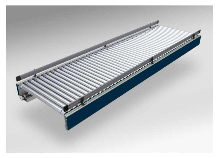
The lineshaft conveyor is a simple and very popular solution for transporting loads. The system requires a small number of drives, which significantly reduces the cost of the conveyor. One gearmotor can drive a line up to 15 meters long.
