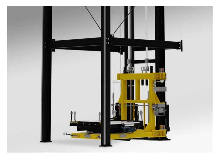
Pallet conveyors make it possible to transport large items such as cartons and pallets. The pallet system minimizes the time needed to transport goods between different areas of the warehouse. By using an elevator, we can optimize the flow of goods through several floors.
