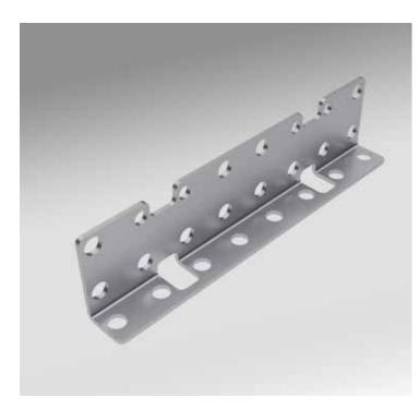
The standard module connectors are made of thick galvanized sheet metal. They allow for the quick and solid connection of the conveyor modules. Each joining of modules requires two pieces of the connectors.
