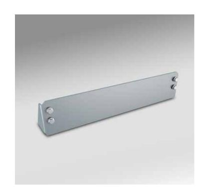
The stop plate is used to block packages at the ends of gravity conveyors. Thanks to this element we can use gravity conveyor as a buffering element. The stop plate is attached to the upper surface of the conveyor side profiles.
