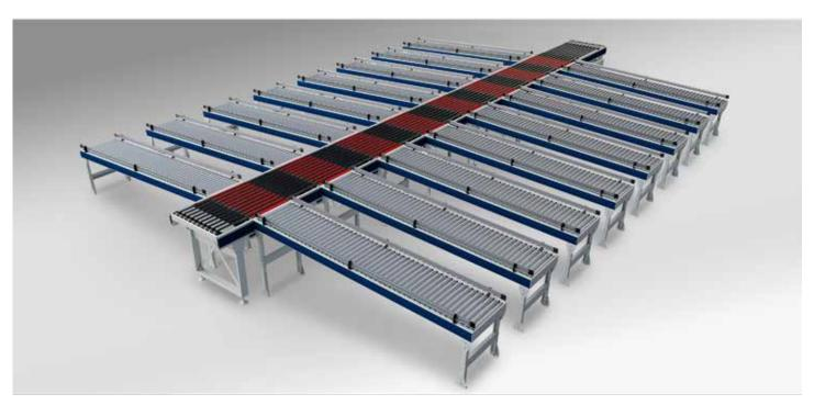
Narrow Belt Sorter uses a set of narrow straps to carry the product over the sorter's surface. In addition, the sorter is equipped with high-friction rollers to enable the dropping of goods. They allow the goods to be picked up from the conveyor for redirection under the 90° to the right or left. The continuous contact of the belt with the product ensures maximum guidance accuracy, which affects the sorting reliability.
